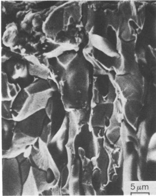
Figure 7 SEM fractograph of the outer and mechanically less-compact part of a boride coating grown in 15 h at 850^\circ\text{C} on an Fe-C-5.65 wt% Cr alloy.
